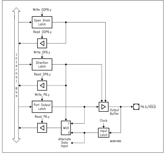
Figure 6-19 Block Diagram of Pin P6.5 (HOLD)
