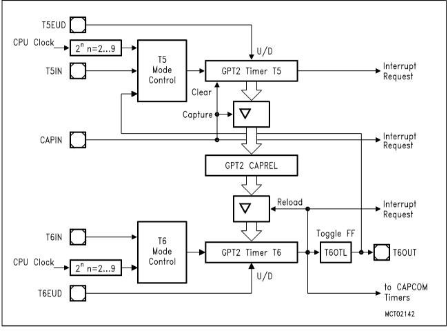
Figure 9-12 GPT2 Block Diagram
