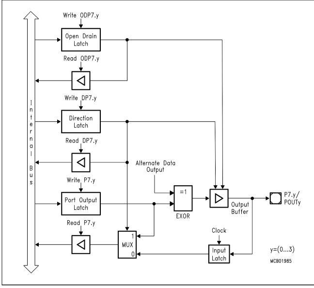
Figure 6-21 Block Diagram of Port 7 Pins P7.3...P7.0
