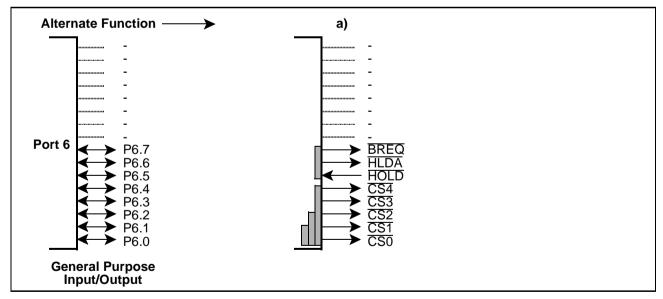
Figure 6-17 Port 6 IO and Alternate Functions
