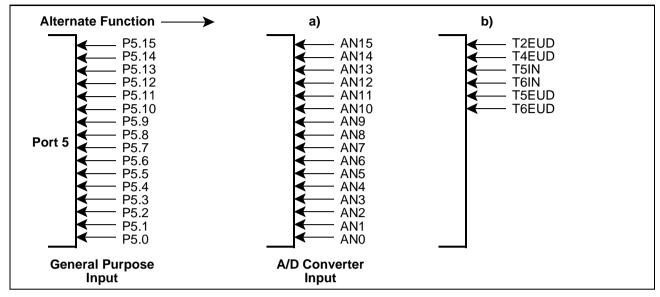
Figure 6-15Port 5 IO and Alternate Functions
