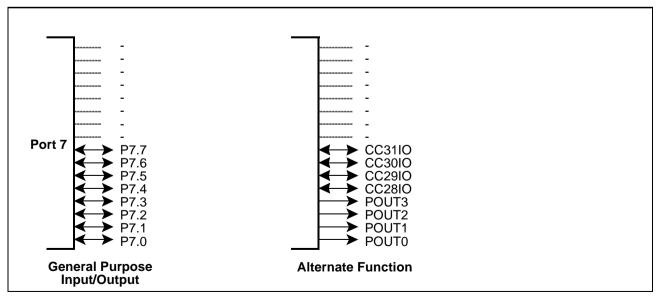
Figure 6-20Port 7 IO and Alternate Functions
