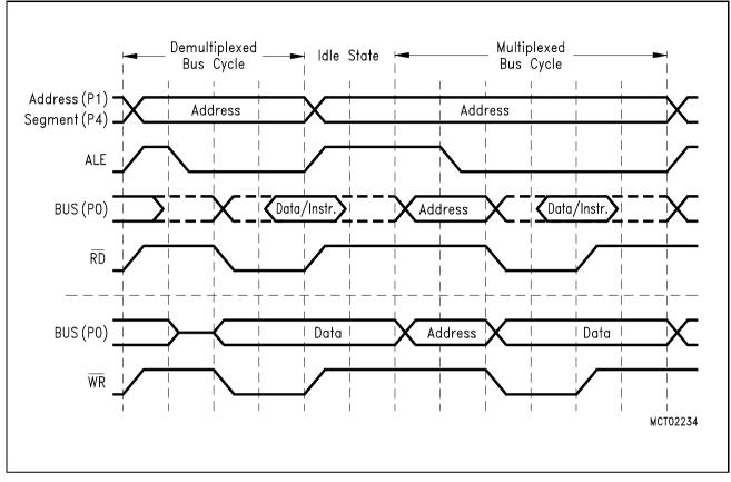
Figure 8-4 Switching from Demultiplexed to Multiplexed Bus Mode
