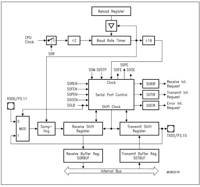
Figure 10-2 Asynchronous Mode of Serial Channel ASC0
