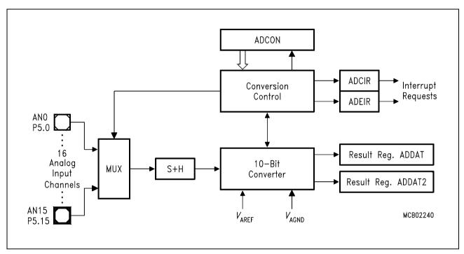
Figure 16-2 Analog / Digital Converter Block Diagram
