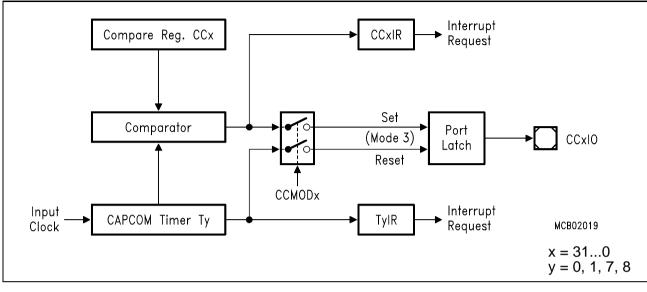
Figure 14-8 Compare Mode 2 and 3 Block Diagram
