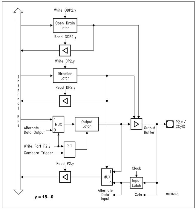
The pins of Port 2 combine internal bus data and alternate data output before the port latch input.
