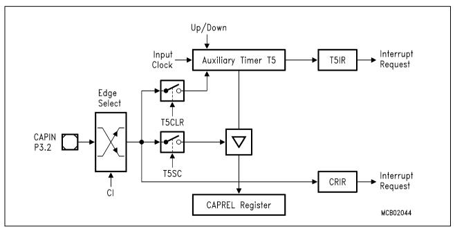
Figure 9-18 GPT2 Register CAPREL in Capture Mode
