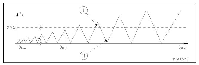
Figure 13-3Baudrate deviation between host and C167
