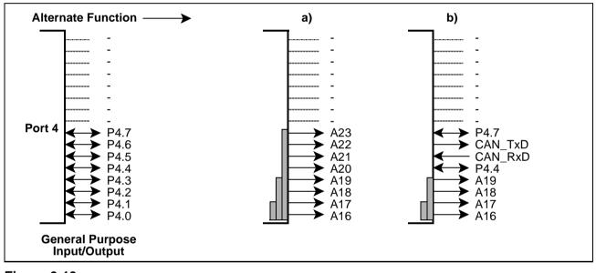
Figure 6-13 Port 4 IO and Alternate Functions
