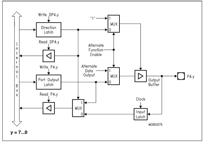
Figure 6-14 Block Diagram of a Port 4 Pin
