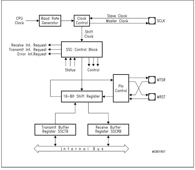
Figure 11-2 Synchronous Serial Channel SSC Block Diagram
