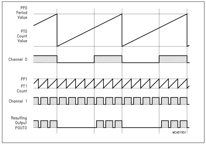
Figure 15-5 Operation and Output Waveform in Burst Mode
