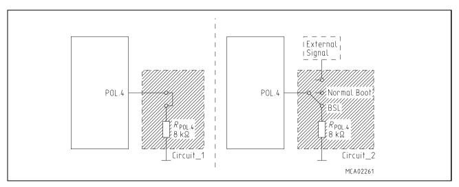
Figure 13-2 Hardware Provisions to Activate the BSL
