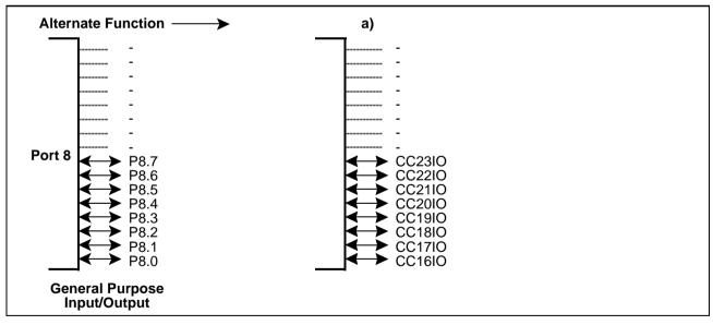
Figure 6-23 Port 8 IO and Alternate Functions
