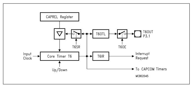
Figure 9-19 GPT2 Register CAPREL in Reload Mode
