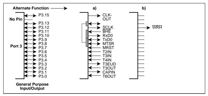
Figure 6-10 Port 3 IO and Alternate Functions
