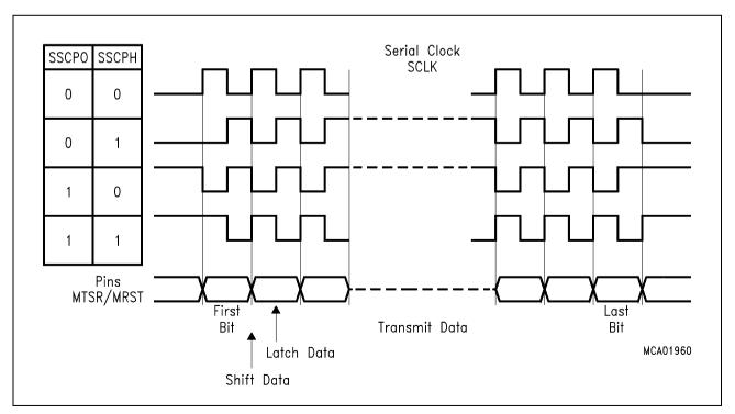
Figure 11-3 Serial Clock Phase and Polarity Options
