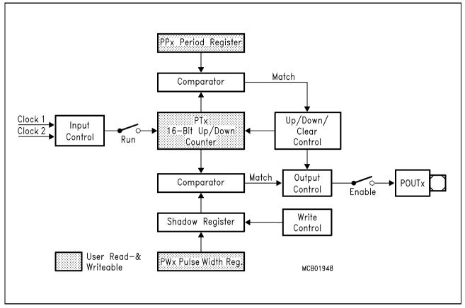
Figure 15-2 PWM Channel Block Diagram
