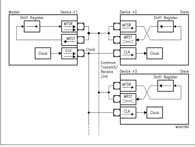
Figure 11-5 SSC Half Duplex Configuration
