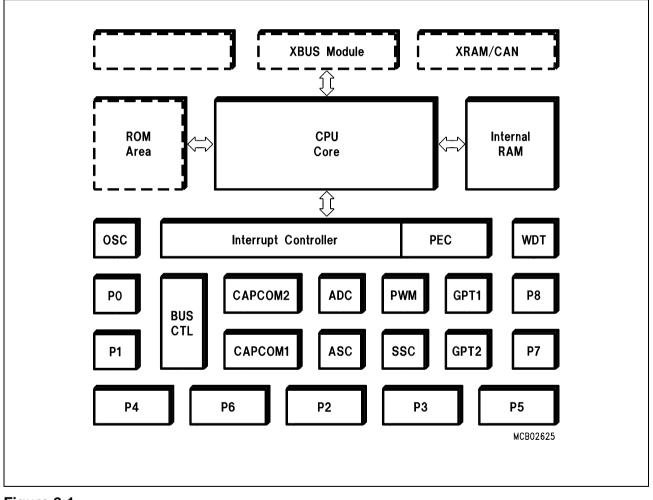
Figure 2-1 C167 Functional Block Diagram
