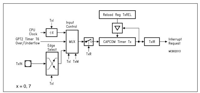
Figure 14-3 Block Diagram of CAPCOM Timers T0 and T7
