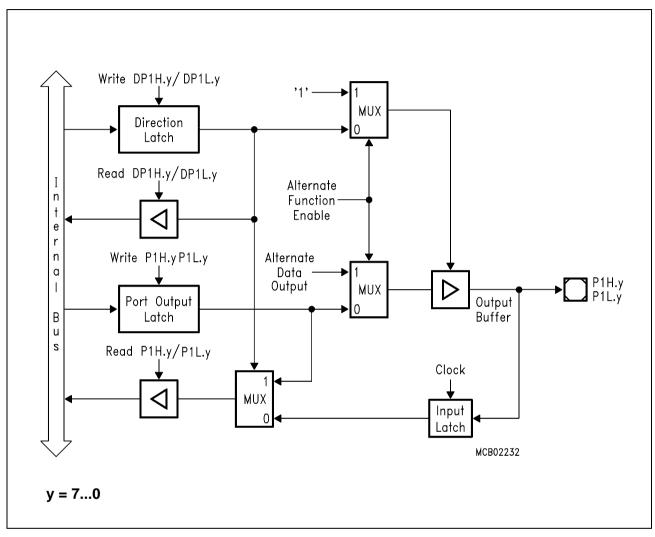
Figure 6-7 Block Diagram of a PORT1 Pin
