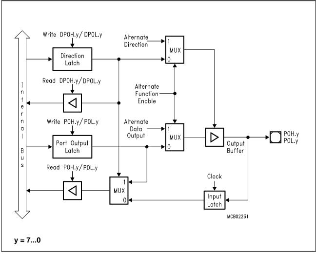
Figure 6-5 Block Diagram of a PORT0 Pin
