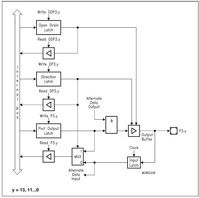
Figure 6-11 Block Diagram of a Port 3 Pin with Alternate Input or Alternate Output Function
