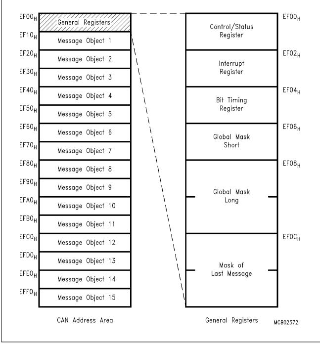
Figure 23-2 CAN Module Address Map
