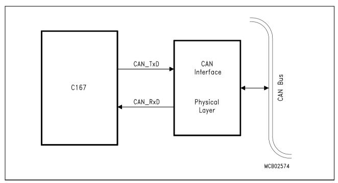
Figure 23-5 Connection to the CAN Bus
