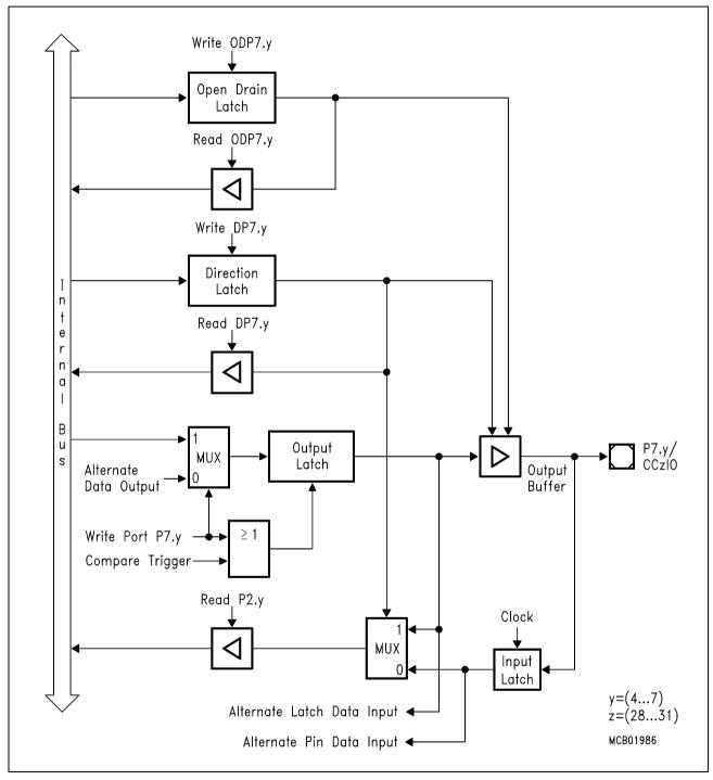
Figure 6-22 Block Diagram of Port 7 Pins P7.7...P7.4
