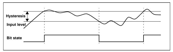
Figure 6-3 Hysteresis for Special Input Thresholds
