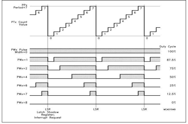
Figure 15-3 Operation and Output Waveform in Mode 0
