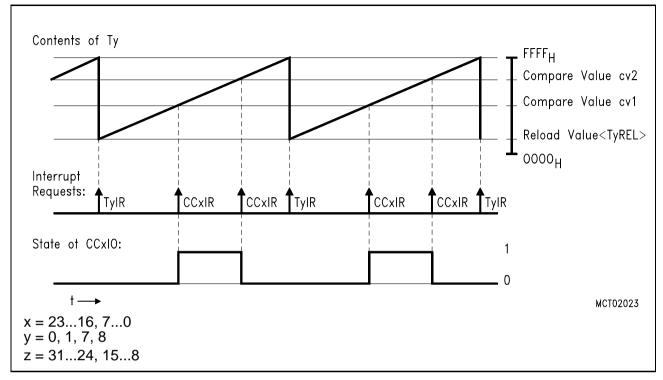
Figure 14-11 Timing Example for Double-Register Compare Mode
