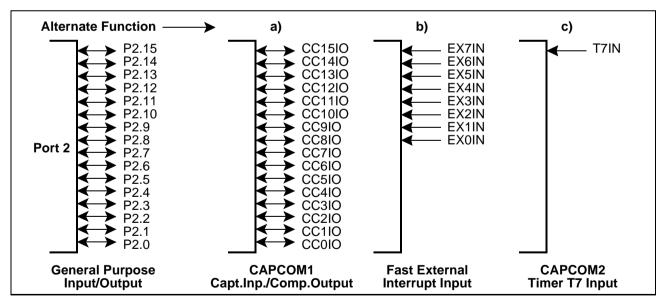
Figure 6-8 Port 2 IO and Alternate Functions
