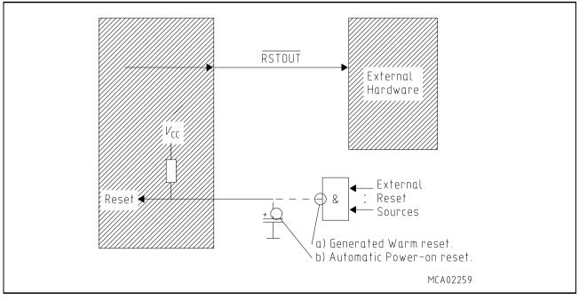
Figure 17-1 External Reset Circuitry
