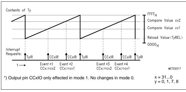
Figure 14-7 Timing Example for Compare Modes 0 and 1
