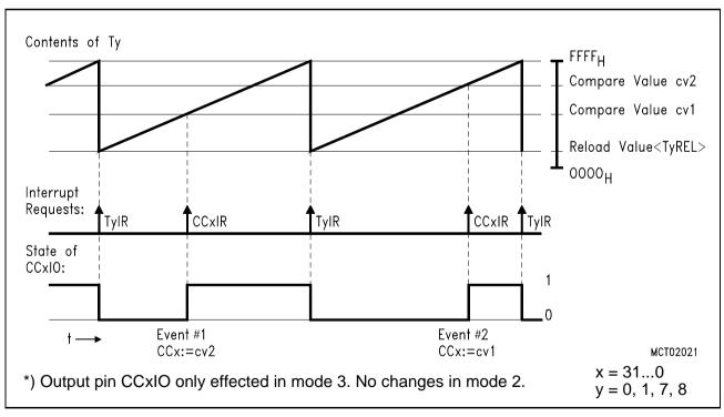
Figure 14-9 Timing Example for Compare Modes 2 and 3
