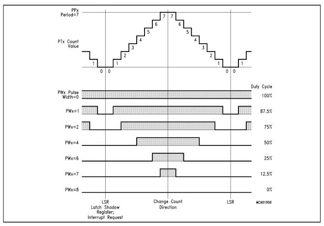
Figure 15-4 Operation and Output Waveform in Mode 1
