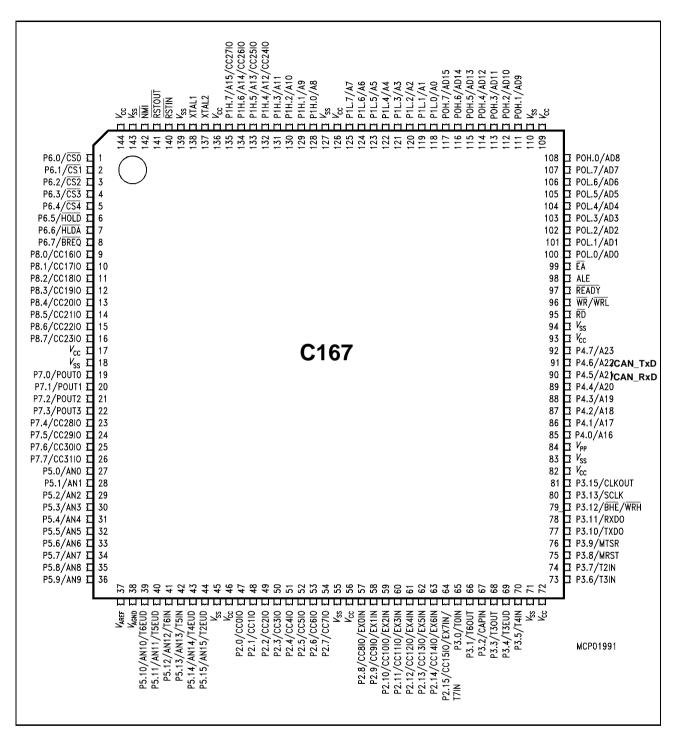
Figure 22-1 Pin Description for C167, P-MQFP-144 Package
