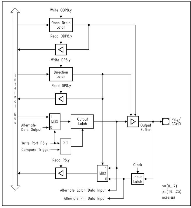
Figure 6-24 Block Diagram of Port 8 Pins
