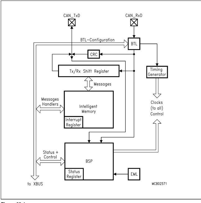
Figure 23-1 CAN Controller Block Diagram
