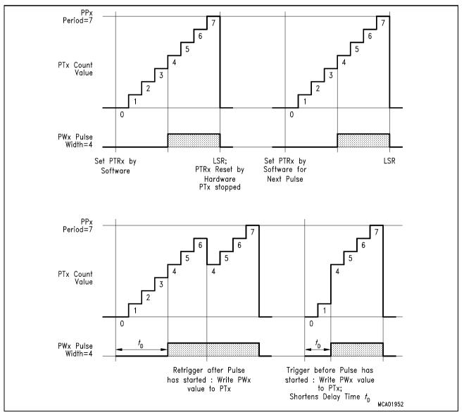
Figure 15-6 Operation and Output Waveform in Single Shot Mode
